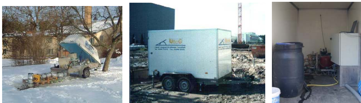
Figure 2: Swedish TRT rig similar to the original one (“TED”) from 1995, on site and coupled to a BHE (left, photo: Hellström); the first UBeG “GeRT” of 1999 on site at DFS Langen (centre) and its interior with the heating unit in the background and the control box to the right (right)
