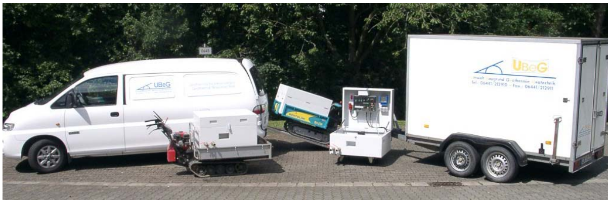
Figure 11: Some GeRT test equipment developed and used by UBeG GbR (the original GeRT trailer to the right, now equipped with a generator for use independent from the grid)
