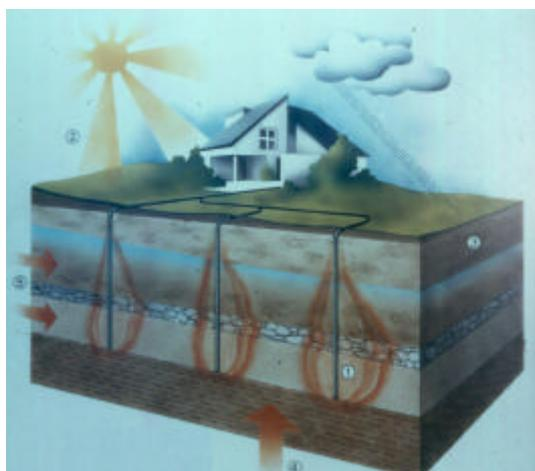
Figure 2: Principle of Ground Source Heat Pump System
