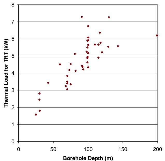
**Figure 6: Thermal load for TRT versus borehole depth for a number of tests performed in 1999-2006**
