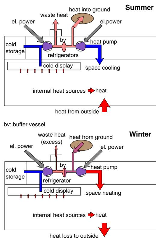
**Figure 2: Schematic of a “total heating and cooling” geothermal system for standardized supermarket (from IGEIA D10-DE, 2008)**
