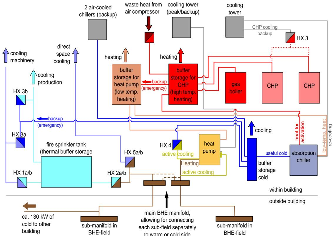
**Figure 17: Simplified schematic of the Leica energy system**
