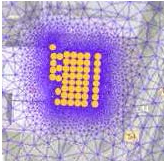
**Figure 13: Central part of the FE-grid for simulation of the Limburg BHE installation, showing the pattern of the 50 BHE**
