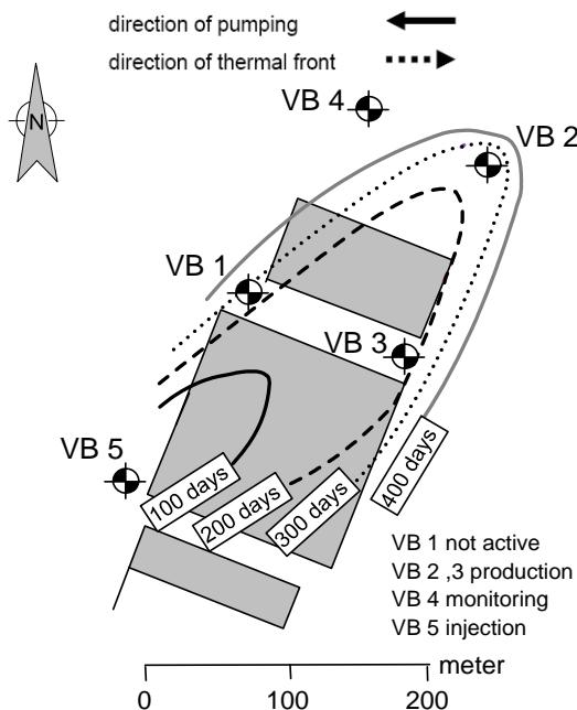
**Figure 12: Travelling time of the thermal front from injection well VB5 after measurements in the period 2007-2011**
