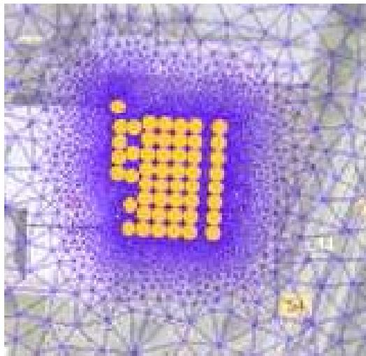
**Figure 13: Central part of the FE-grid for simulation of the Limburg BHE installation, showing the pattern of the 50 BHE**
