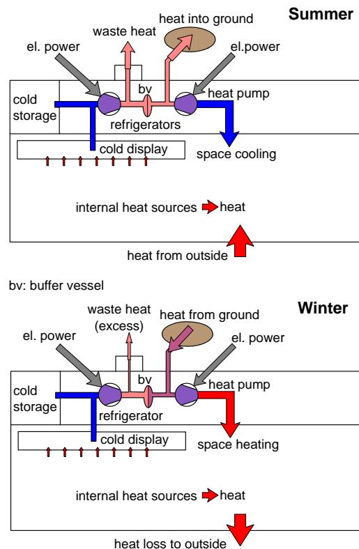
**Figure 2:** Schematic of a “total heating and cooling” geothermal system for standardized supermarket (from IGEIA D10-DE, 2008)
