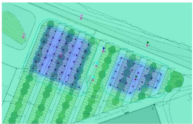
**Figure 15: Numerical simulation of temperature influence of Leica BHE field, situation after 10 years at the end of the heating season**
