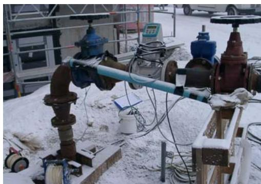
**Figure 9: A production well at the Regensburg site with measuring device, during the pumping test with all wells coupled, February 2006**
