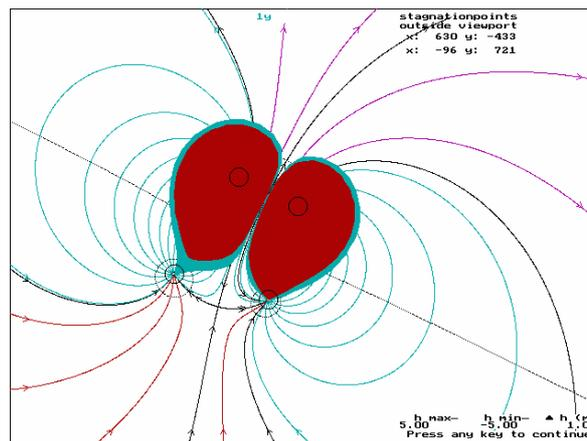
**Figure 10: Thermal front prediction of 2005 using CONFLOW, with well VB4 intended as injection well; the width of the graph represents 800 m**
