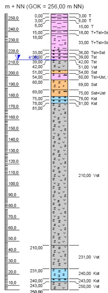
**Figure 8: Lithological cross-section of 250-m-borehole for BHE in Weilburg: Devonian shale (Tst), sandstone (Sst), and conglomerate (Vst, local name “Schalstein”), with few limestone banks (Kst)**
