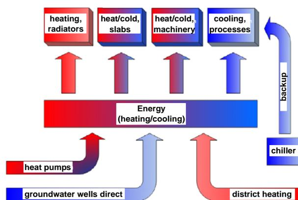
**Figure 11: Schematic of thermal energy supply for Regensburg plant**
