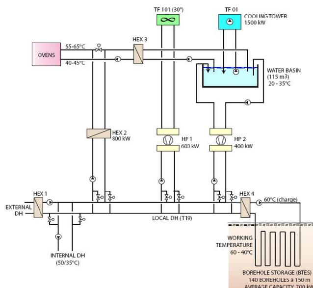
**Figure 4: Schematic of BTES plant in Swedish feasibility study (from IGEIA D10-SE, 2008)**
