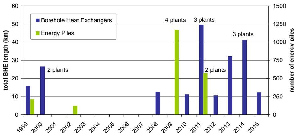
**Figure 4: Construction of very large geothermal heat pump plants in Germany (more than 10 km BHE, and for energy piles more than 350 kW system capacity).**
