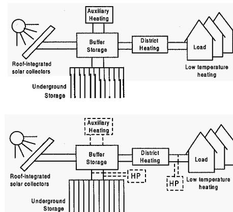
*Figure 2: Solar heat storage with direct (above) and heat-pump-supported (below) unloading of the store*
