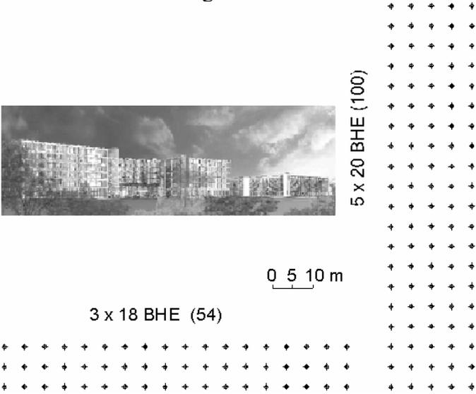
Fig. 8: Layout of the two BHE fields for the office building in Langen, with the architect’s impression of the building to show its location in regard to the BHEs
