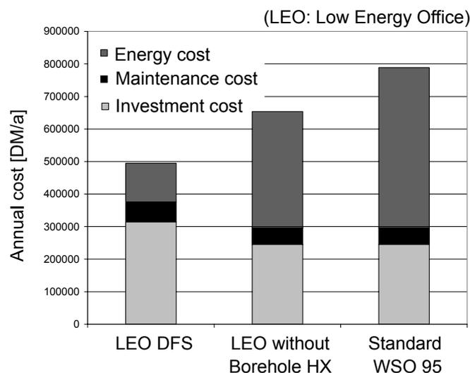
Fig. 12: Annual cost comparison for heating and cooling the German Air Traffic Control (DFS) headquarters (after [9])
