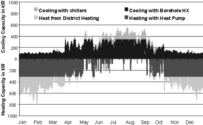
Fig. 9: Heating and cooling demand for the German Air Traffic Control (DFS) headquarters, data from simulation
