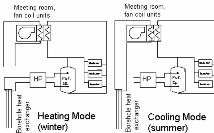
Fig. 4: *Schematic of the first experiment with direct cooling from BHE, GSHP plant for heating and cooling in the office building of Helmut Hund GmbH (from [4])*
