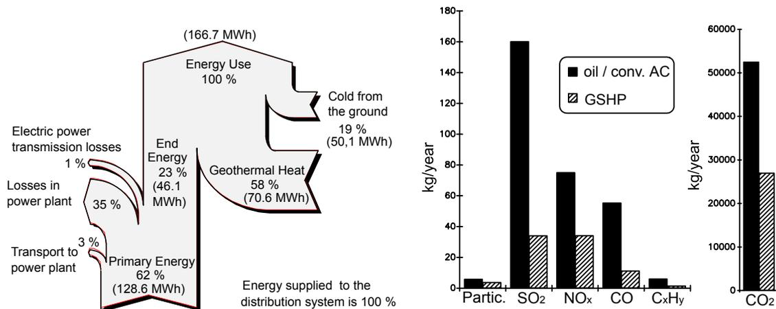
Fig. 7: left: Energy flow for UEG plant, Wetzlar, in 1995/96, starting from primary energy; the values given for electricity production are from a utility report
