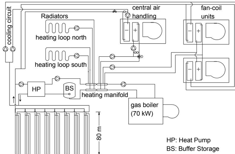
Fig. 6: Schematic of the GSHP plant for heating and cooling in UEG building, Wetzlar
