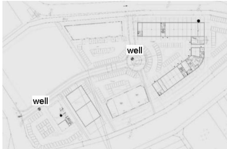
*Fig. 15: Plan of the commercial area in Hainburg to be heated and cooled by GSHP*
