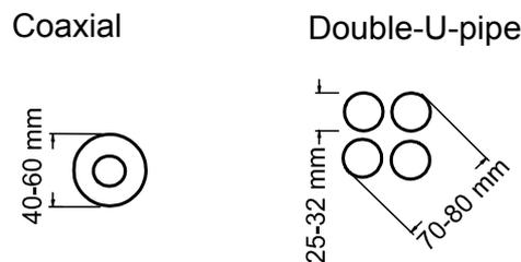
Fig. 4: *Cross-section of typical BHE, as used in Schwalbach*
