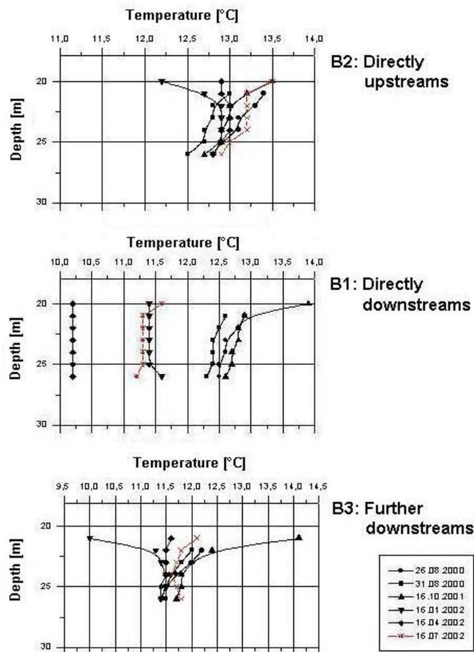
Fig. 11: *Monitoring of the impact of the BHE-field on groundwater temperature*
