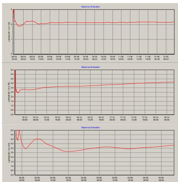
**Figure 5: Sequential evaluation of TRT showing a stable result (top), a steady increase of thermal conductivity over test time (groundwater influence, centre) and erratic variations (e.g. due to power fluctuations, bottom), from Sauer & Sanner (2011)**
