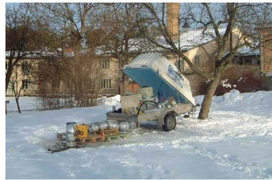
**Figure 1:** Swedish test rig, coupled to a borehole heat exchanger
