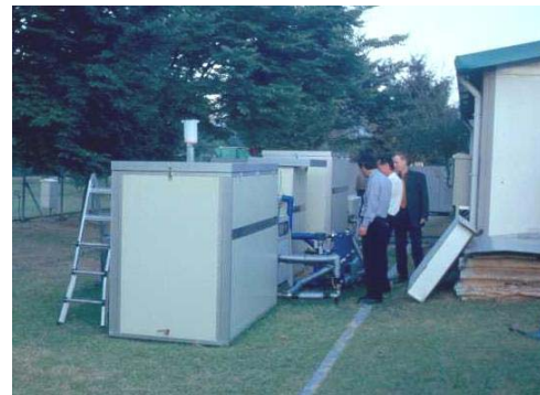
Figure 5: Experimental heat pump made by HP System Tech, with hot water- and ice-storage tanks (photo Sanner, Oct. 2003)
